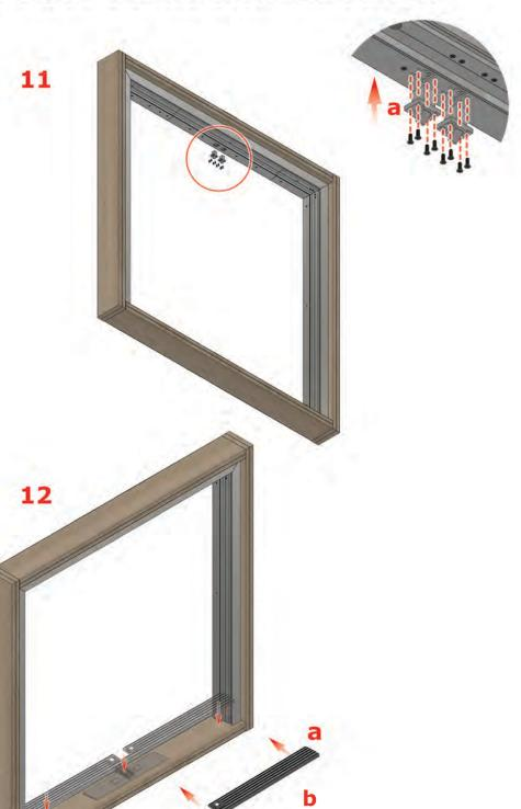
**12.** Slide Threshold (a) and stainless steel plate (b) into door opening.
